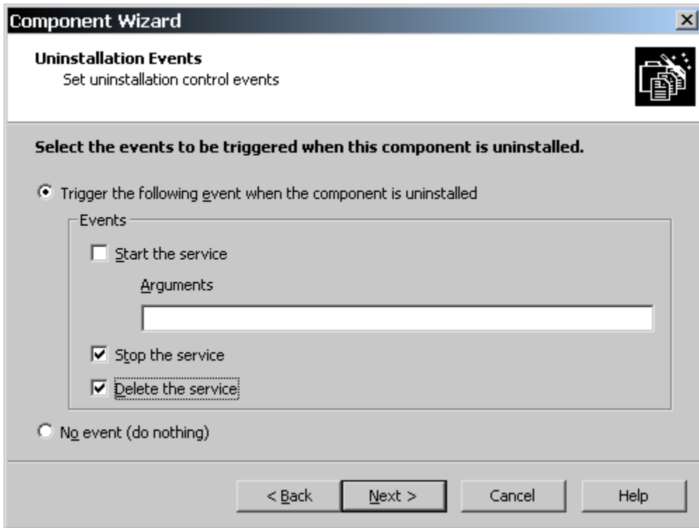
Figure 14-27: Specifying the events to occur during the uninstallation of an NT service.
