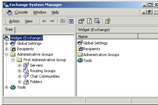
FIGURE 7.2 System Manager showing administrative and routing groups
