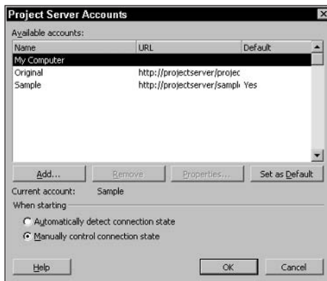
Figure 20-1: Use this dialog box to add a Project Server logon account and to specify connection state detection options.
