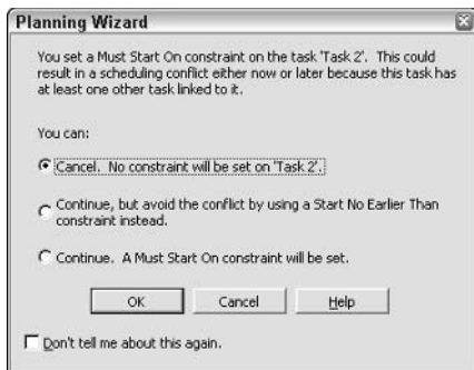
Figure 9-6: The Planning Wizard appears by default when you apply a constraint that is likely to lengthen your project schedule.
