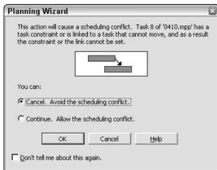
Figure 4-19: Multiple dependencies or a combination of dependencies and constraints can cause conflicts in timing.
