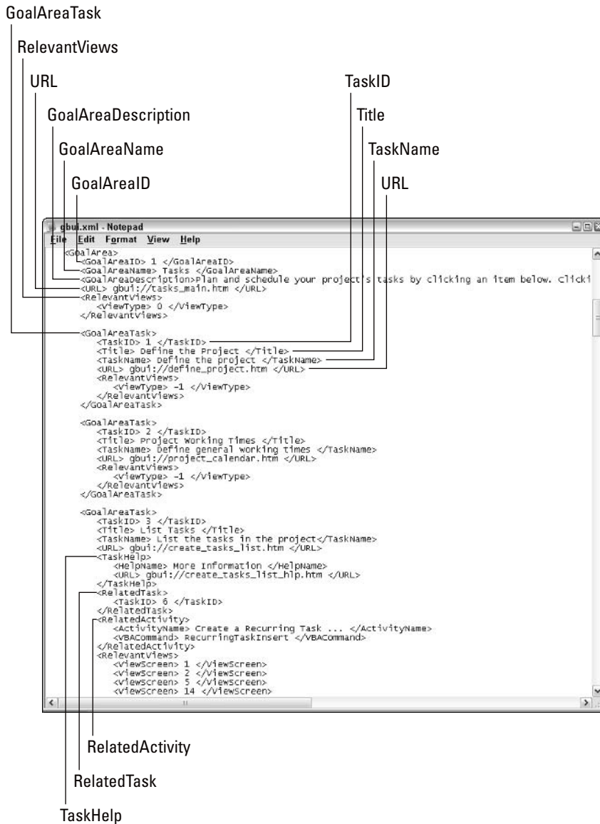
Figure 25-27: The GoalArea element defines the tasks that appear in the Project Guide side panes.
