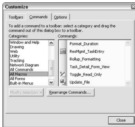
Figure 24-6: From the Commands tab of the Customize dialog box, you can add macros as buttons to toolbars.
