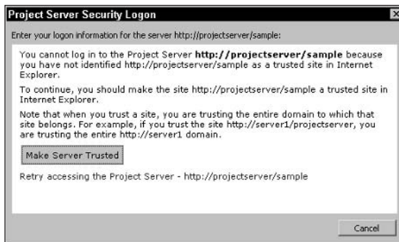
Figure 20-4: Make your Project Server site a trusted site the first time you log on.
