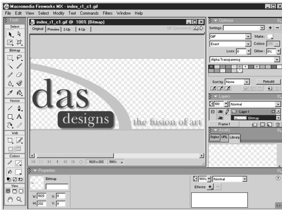
FIGURE 12-1 When you have an image with large areas of solid color, GIF is the ideal export format.
