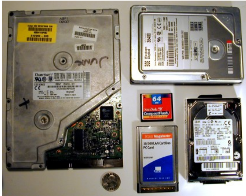
The five most popular internal form factors for PC hard disks. Clockwise from the left: 5.25", 3.5", 2.5", PC Card and CompactFlash.
