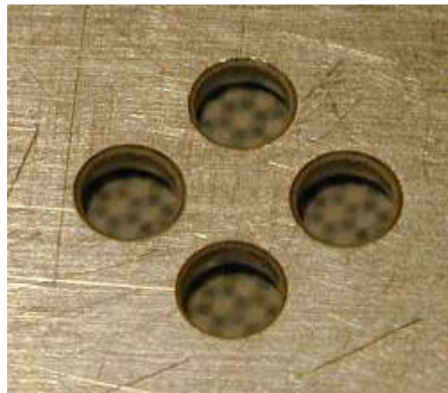
Closeup shot of the breather holes in the top of a hard disk case. Part of the breather filter can be seen just under the holes.
