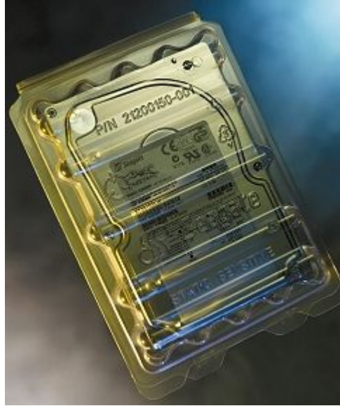
A Seagate "SeaShell", containing a Cheetah SCSI drive.
