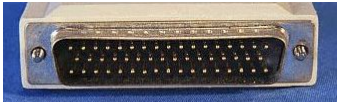
A male DD-50 SCSI connector. Note the "D-shaped" metal shell around the pins.
