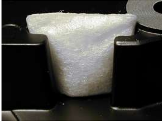
A recirculating filter in the top cover of a consumer-grade hard disk.
