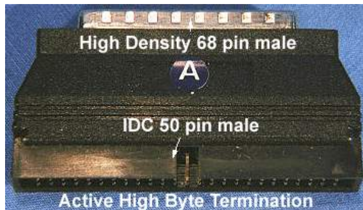
A wide/narrow adapter that includes high byte termination.
