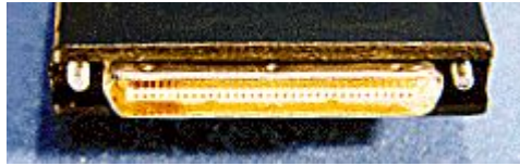
A male 68-pin VHDCI connector.
