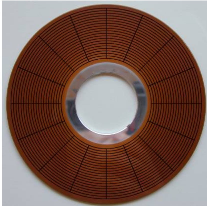
A platter from a 5.25" hard disk, with 20 concentric tracks drawn over the surface. Each track is divided into 16 imaginary sectors.
