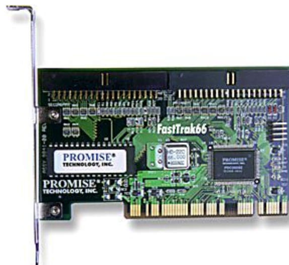
A PCI-bus-based, IDE/ATA hard disk RAID controller, supporting levels 0, 1, and 01. (Promise's popular FastTrak 66.)
