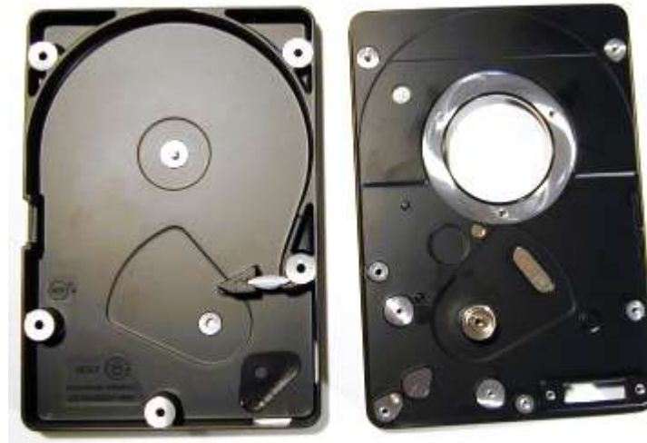
Cover (left) and base casting (right) of a consumer-grade IDE/ATA hard disk drive. All the components have been removed to show the detail (except the recirculating filter is still in place on the cover... Oops! You can see a proper picture of that filter here .)
