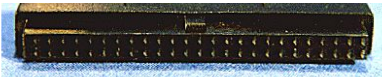
Male (above) and female 50-pin regular density internal connectors. Note the gap in the plastic shield around the male connector, and the tab on the female connector, for keying.
