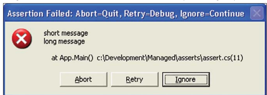
Figure 1: Typical assert shown for Debug.Assert or Debug.Fail . The short and long descriptions are shown on separate lines followed by a stack trace.
