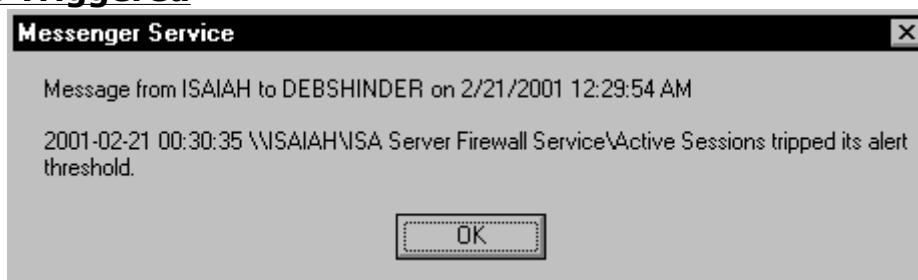
Figure 11.12 A Network Message Is Sent to the Specified Account When the Alert Is Triggered
