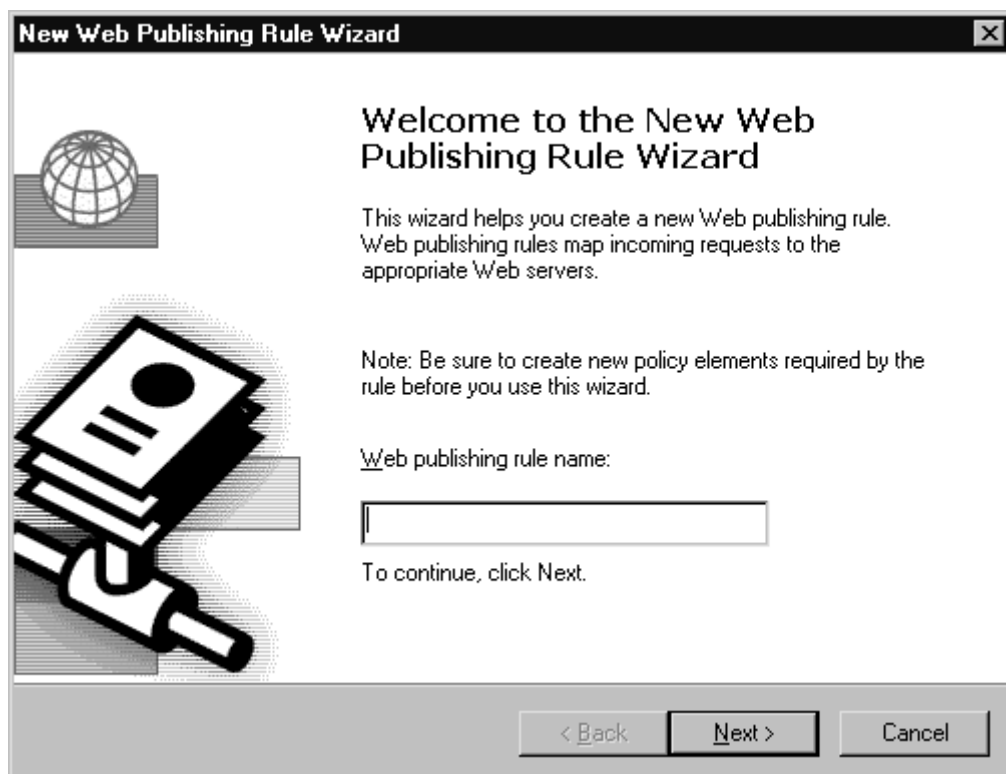
Figure 6.23 New Web Publishing or Server Publishing Rules Are Created with a Wizard
