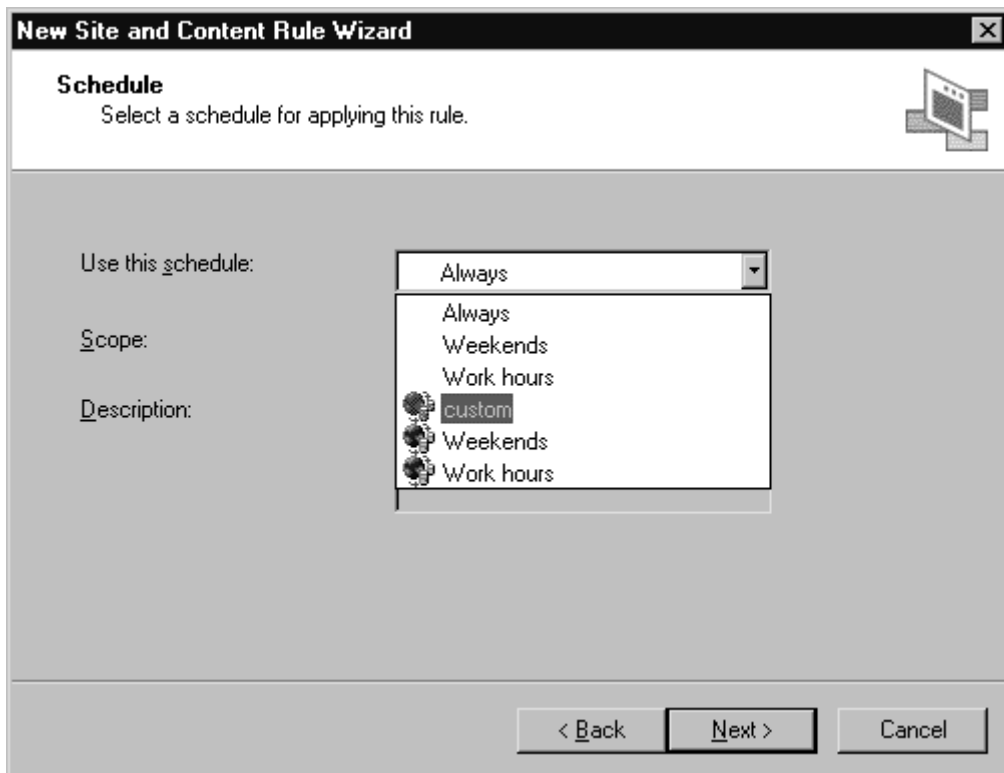
Figure 6.17 The Policy Element Created at the Enterprise Level Is Available to Be Applied to Rules at the Array Level
