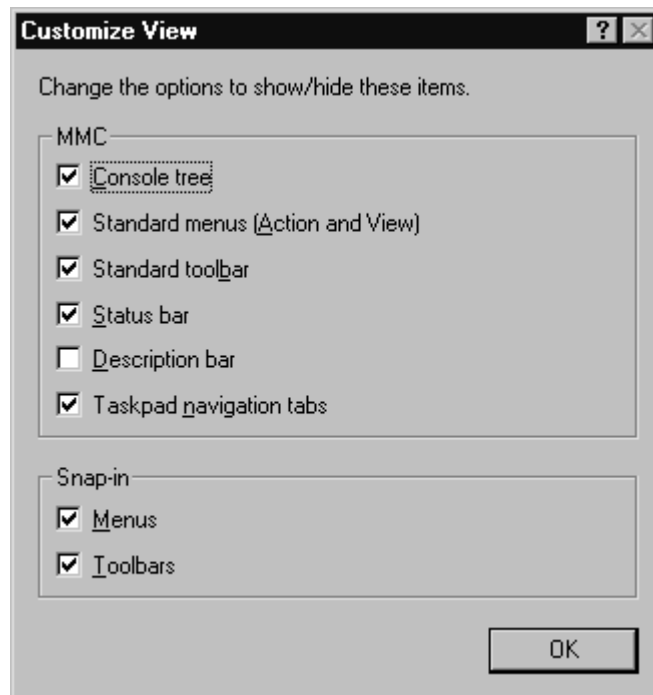
Figure 6.6 You Can Select the MMC Elements You Wish to Display or Hide
