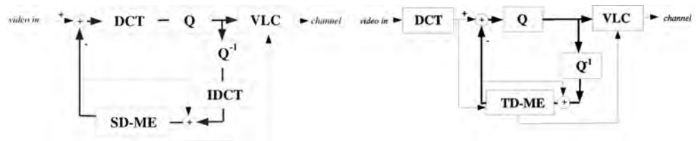
FIGURE 9.2 Different MC-DCT video coder structures: (a) motion estimation/compensation in the spatial domain; (b) motion estimation/compensation completely in the transform (DCT) domain.
