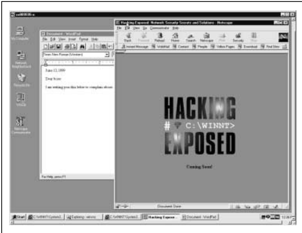
Figure 5-9. WinVNC connected to a remote system. This is nearly equivalent to sitting at the remote computer
