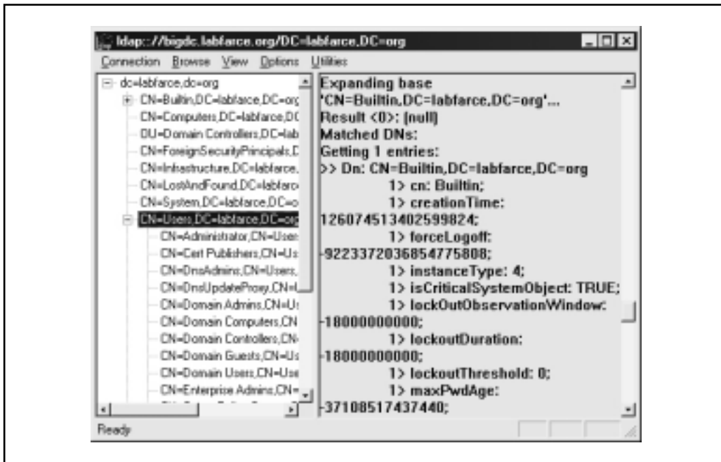
Figure 3-4. The Active Directory Administration Tool, ldp.exe, enumerates Active Directory users and groups via an authenticated connection
