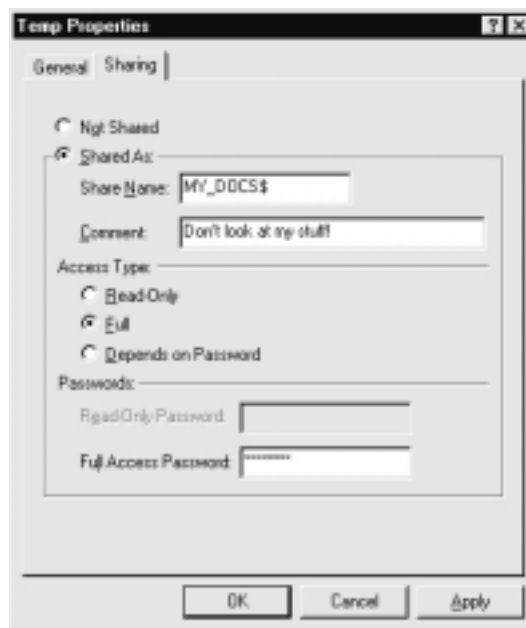
Figure 4-3. Append a $ to the name of a file share to prevent it from appearing in the Network Neighborhood and in the output of many NetBIOS scanning tools
