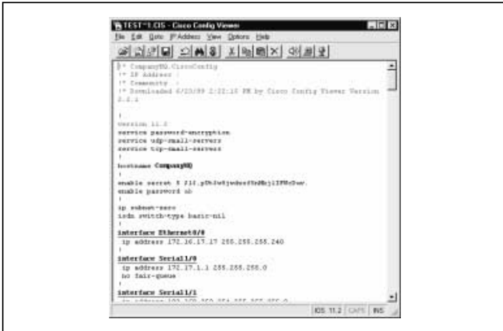
Figure 10-5. Decrypting the Cisco passwords within the configuration file is trivial with SolarWinds' Cisco Config Viewer's password decryptor
