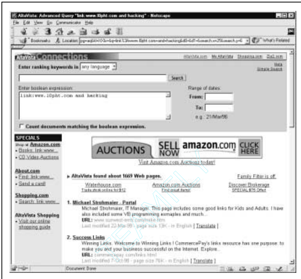
Figure 1-1. With the AltaVista search engine, use the link:www.targetdomain.com directive to query all sites with links back to the target domain
