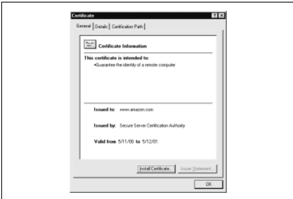
Figure 16-5. A server's SSL certificate is examined in IE. Make sure that this information is as expected when visiting SSL-ized servers
