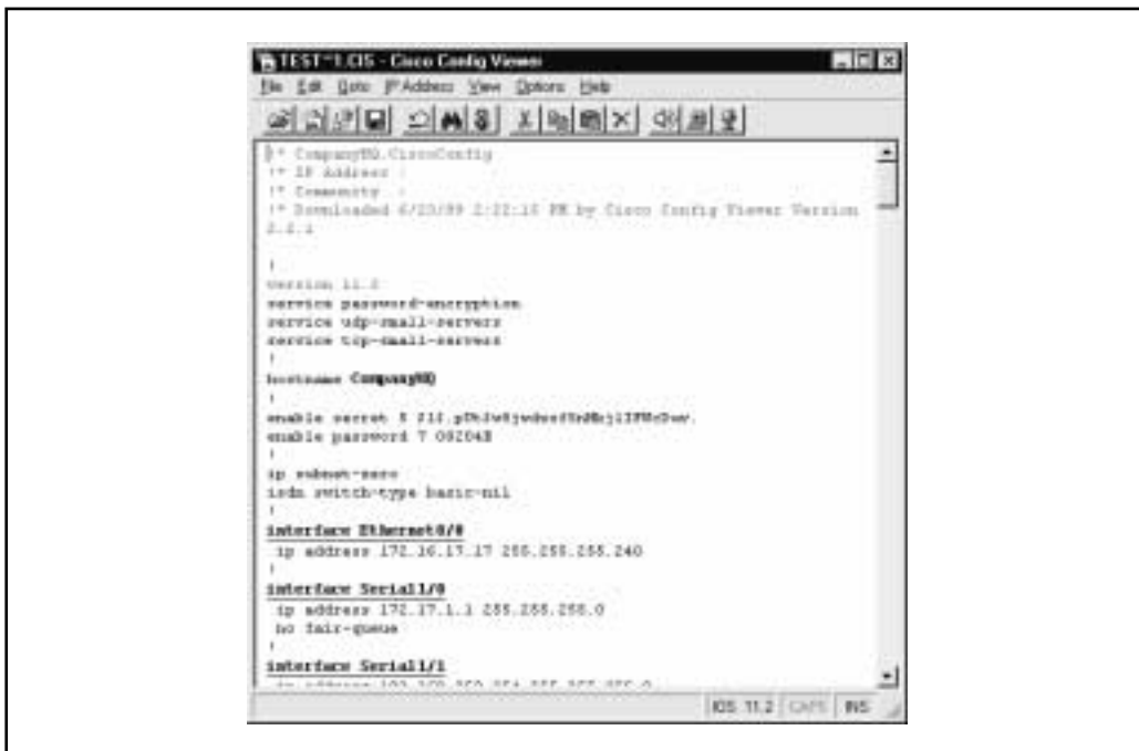
Figure 10-4. SolarWinds' Cisco Config Viewer enables easy download of the Cisco configuration file once the read/write community string is known
