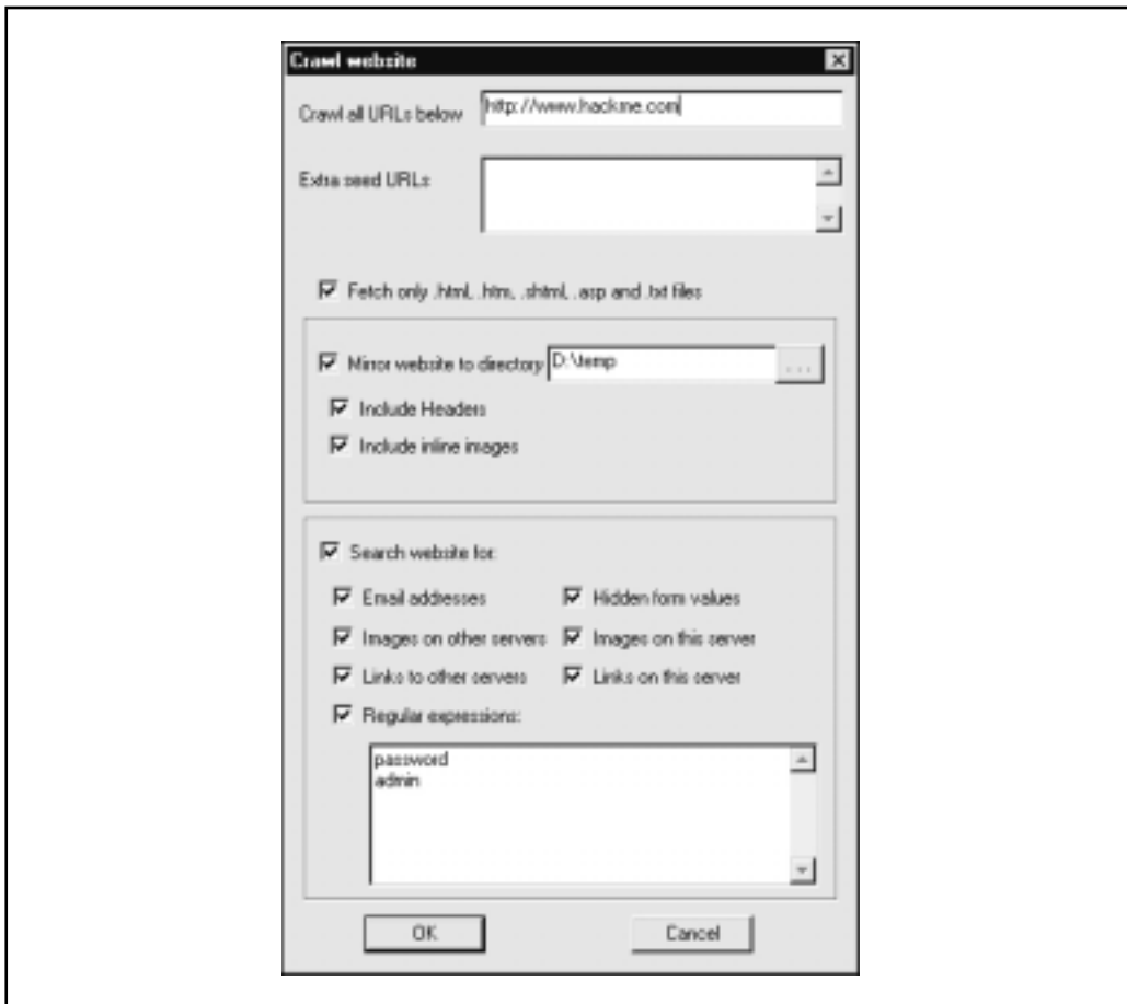
Figure 3-12. Sam Spade’s “Crawl Website” feature makes it easy to parse entire sites for juicy information like passwords
