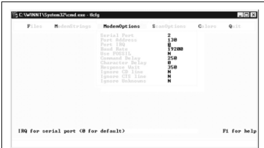
Figure 9-1. Using TLCFG.EXE to enter modem configuration parameters to be used by ToneLoc for wardialing
