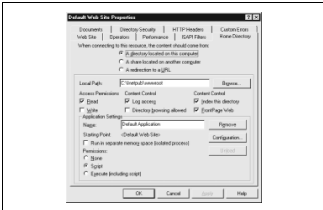
Figure 5-5. The Home Directory tab of a virtual web folder under IIS, showing Execute permissions disabled
