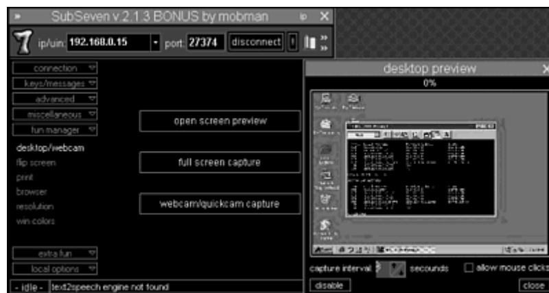
Figure 15.10. The fun manager, which enables the attacker to play some tricks on the victim.
