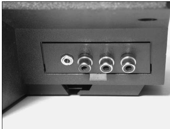
Figure 9.105 The New Video and Audio Connectors, Left to Right: Audio, Composite Video, Luma, and Chroma
