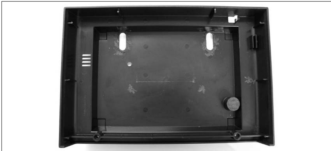
Figure 2.54 Atari 2600 Bottom Housing with Unnecessary Plastic Removed
