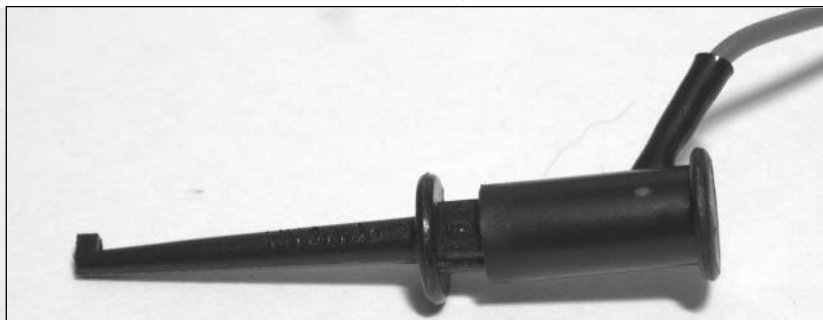
Figure 9.72 Contents of the Atari 5200 Video Upgrade Board: Probe Clip
