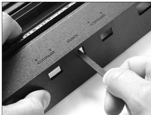
Figure 2.61 Enlarging the Case to Fit the New Power Jack
