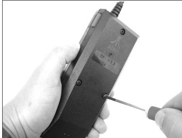
Figure 9.35 Removing the Three Screws from the Back of the 5200 Controller
