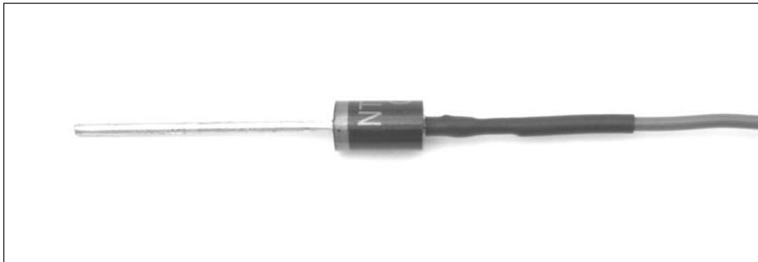
Figure 9.55 Solder the Red Wire the 1N5391G Diode
