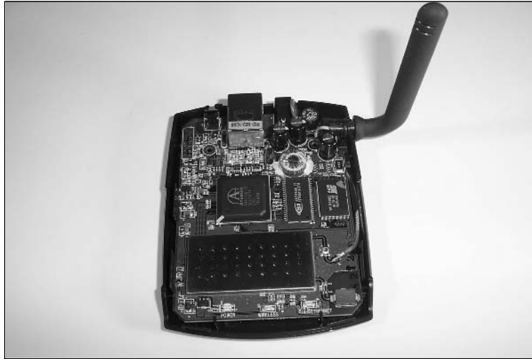
Figure 3.37 Xbox Wireless Adapter with Top Removed
