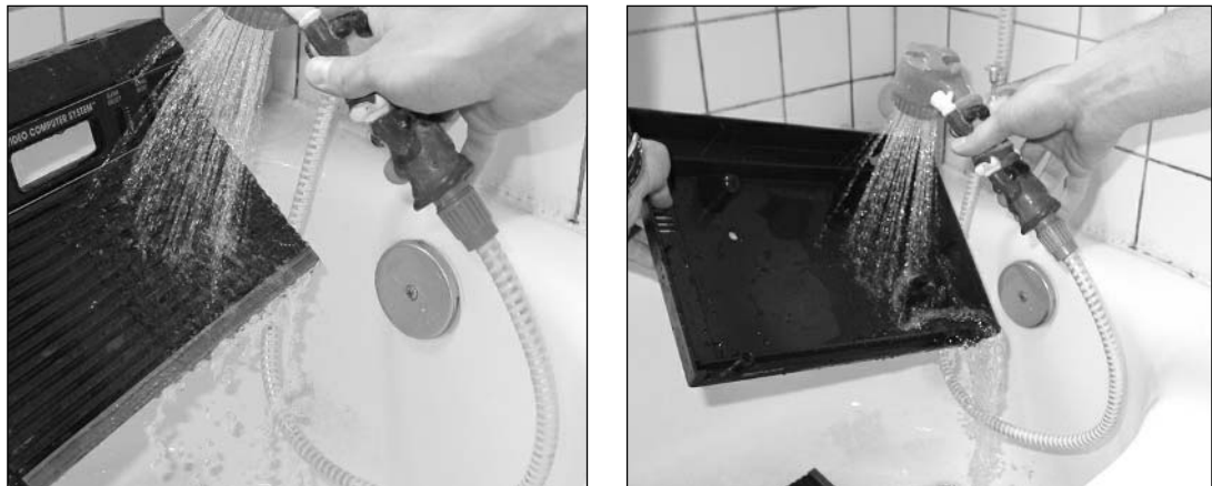
Figure 2.9 Rinsing the Atari 2600's Plastic Housing (Top and Bottom Pieces)
