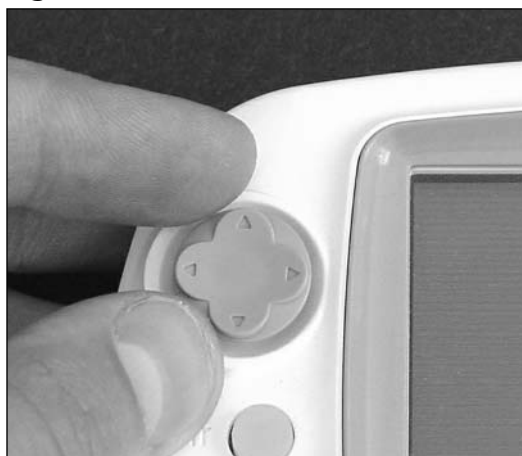
Figure 6.12 Remove the Plastic Directional Joystick, Before and After
