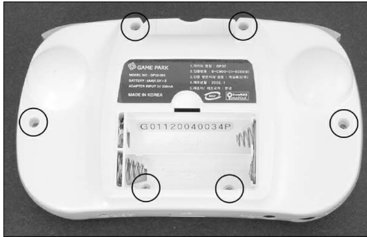
Figure 6.13 Backside of the GP32 Showing Screw Locations
