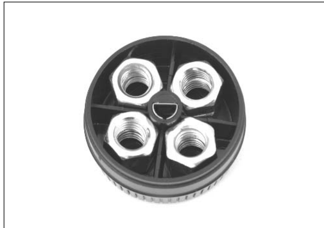
Figure 9.48 Weighing Down the Dial with Hex Nuts
