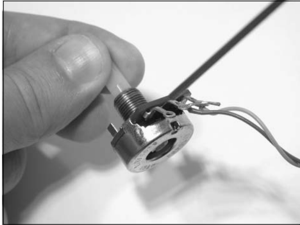
Figure 8.29 Spraying the Contact Cleaner
