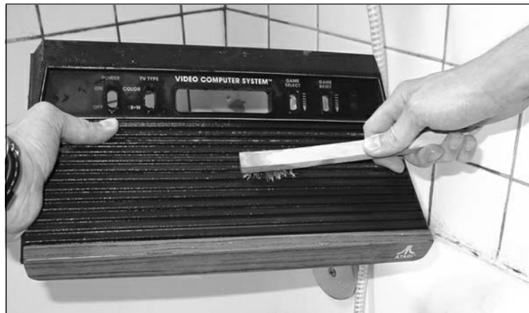
Figure 2.10 Scrubbing the Atari 2600's Plastic Housing
