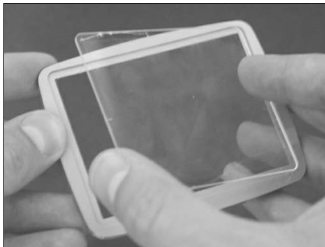
Figure 6.27 Removing the Old Screen Cover from the Plastic Bezel
