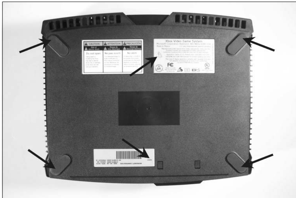
Figure 3.4 The Six Screws Are Hidden Underneath the Labels and Rubber Feet
