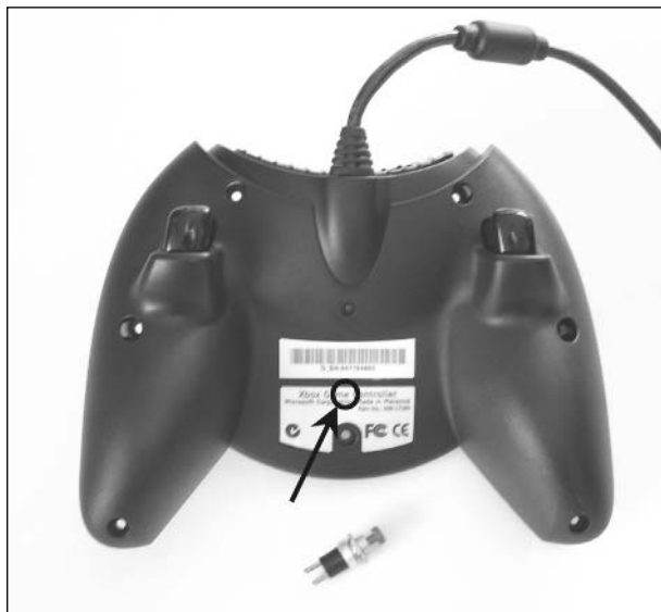
Figure 3.18 Preferred Location for the Reset Button
