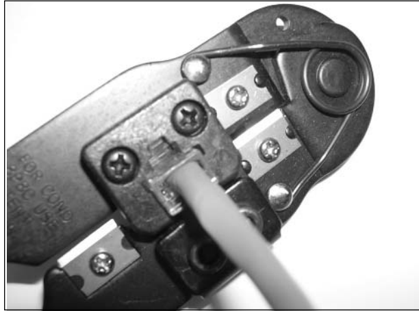
Figure 3.29 Crimping the RJ-45 Plug
