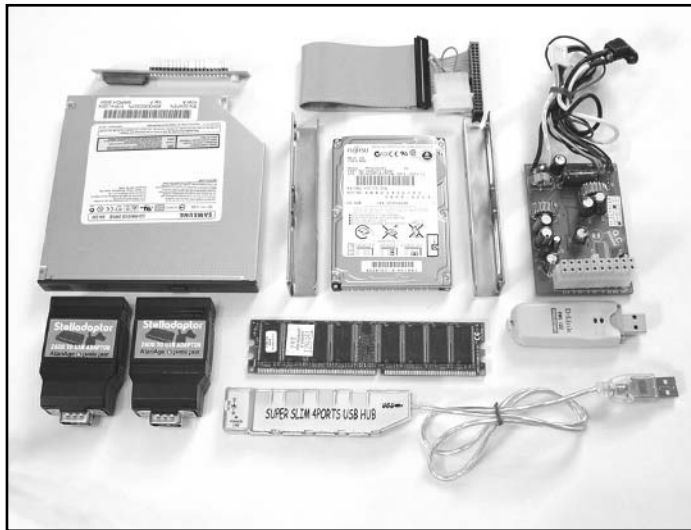
Figure 2.5 Most of the External Components Required for the Atari 2600PC Case Mod
