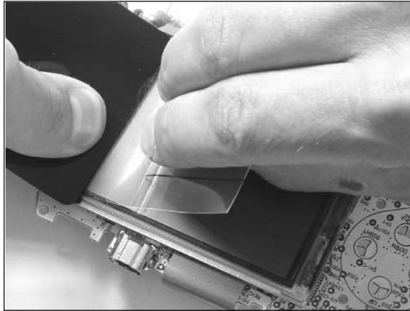
Figure 5.40 Laminating the Antireflective Film to the LCD
