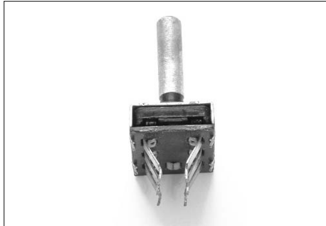
Figure 2.20 Bent Leads of the Momentary Switch to Fit into the S201 Footprint
