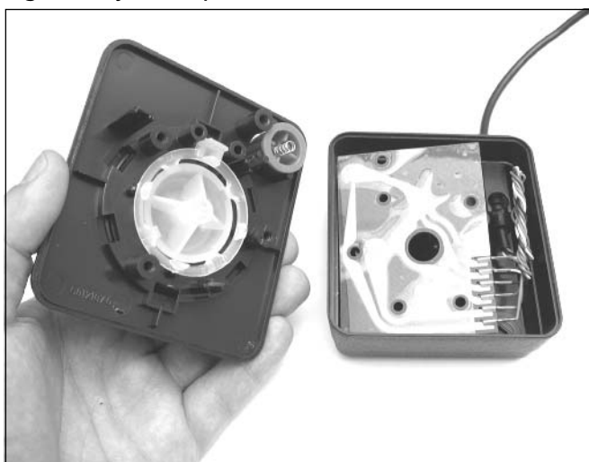
Figure 8.4 Taking the Joystick Apart
