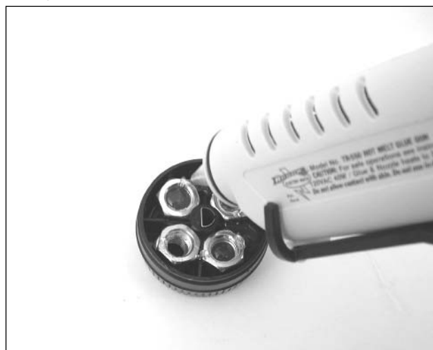
Figure 9.49 Gluing Your Nuts into Place
