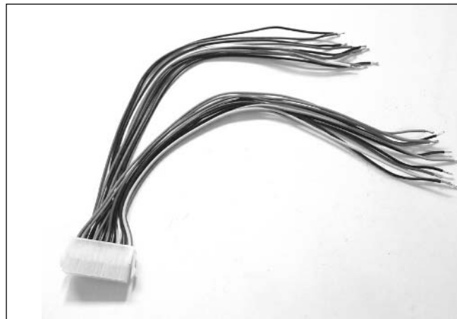
Figure 2.51 ATX Extension Cable Ready to Be Soldered to the Motherboard
