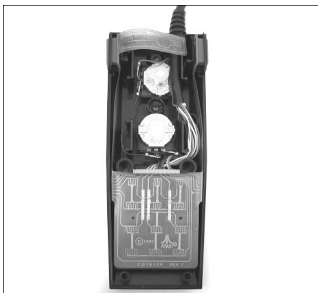
Figure 9.37 Bottom Half of the Atari 5200 Controller
