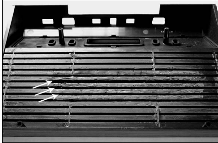
Figure 2.65 The Completed, Modified Atari 2600 Top Housing, with Arrows Denoting Slots for DRAM
