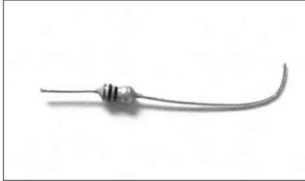
Figure 5.42 Bend and Clip the Resistor
