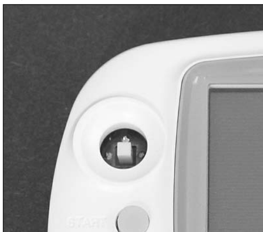
Figure 6.12 Remove the Plastic Directional Joystick, Before and After
