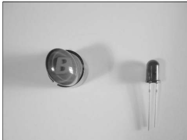
Figure 3.12 The Red "B" Button and Red LED
