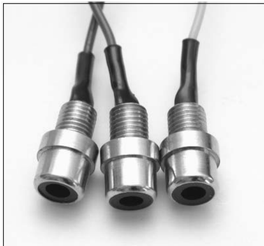
Figure 9.70 Contents of the Atari 5200 Video Upgrade Board: Pre-Wired Video Connectors
