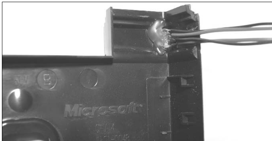
Figure 3.32 Back View of the LEDs Mounted on the Front Panel
