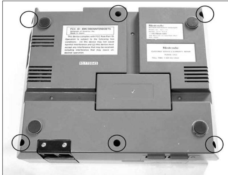
Figure 7.4 The Underside of the Nintendo NES, Showing Screw Locations
