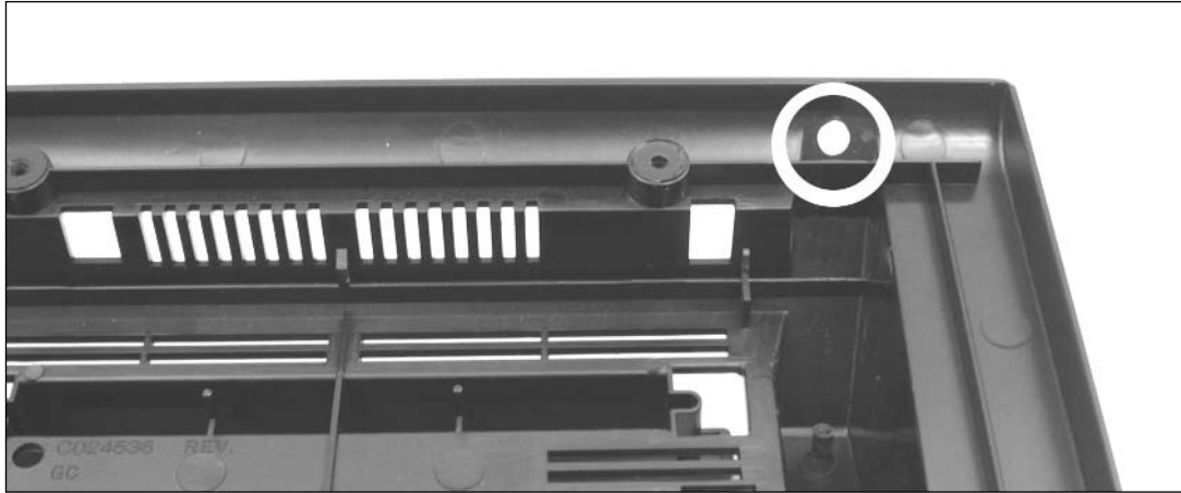
Figure 10.27 Drill a Hole into the Atari 7800 Case for the Phone Jack
