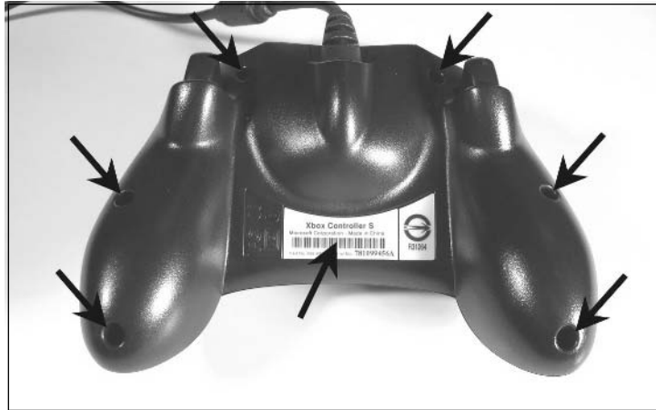
Figure 3.9 The Bottom of the S Controller
