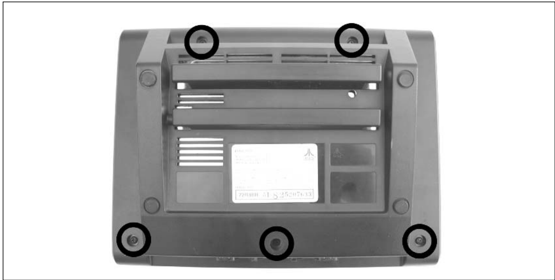
Figure 10.3 Remove the Five Screws
