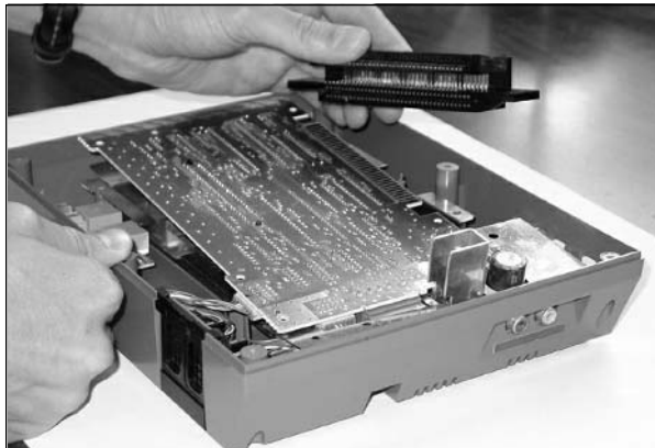
Figure 7.14 The Old 72-pin Cartridge Connector Is Successfully Removed
