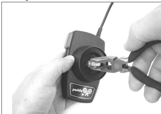
Figure 9.32 Removing the Paddle Nut
