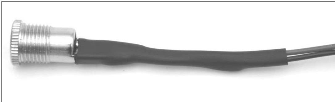
Figure 9.58 Completed View of the Power Cable
