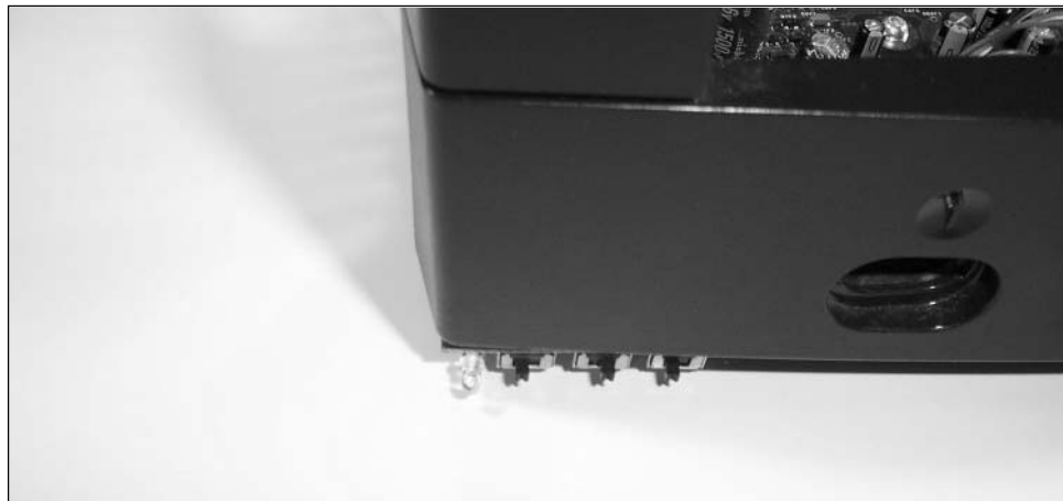
Figure 3.50 Xecuter Switchboard as Seen From the Front of the Xbox
