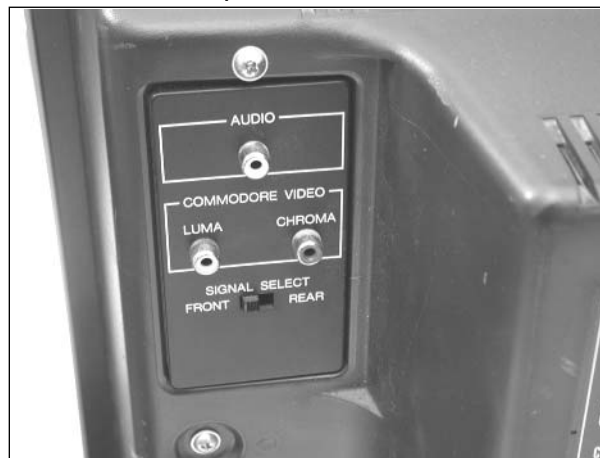
Figure 8.73 Commodore 1702 Rear Input Jacks
