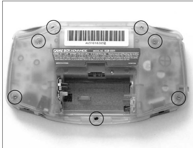
Figure 5.6 Backside of the GBA Showing Screw Locations
