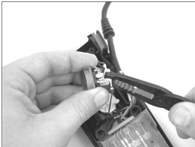
Figure 9.39 Removing Wires from the Upper 5200 Potentiometer
