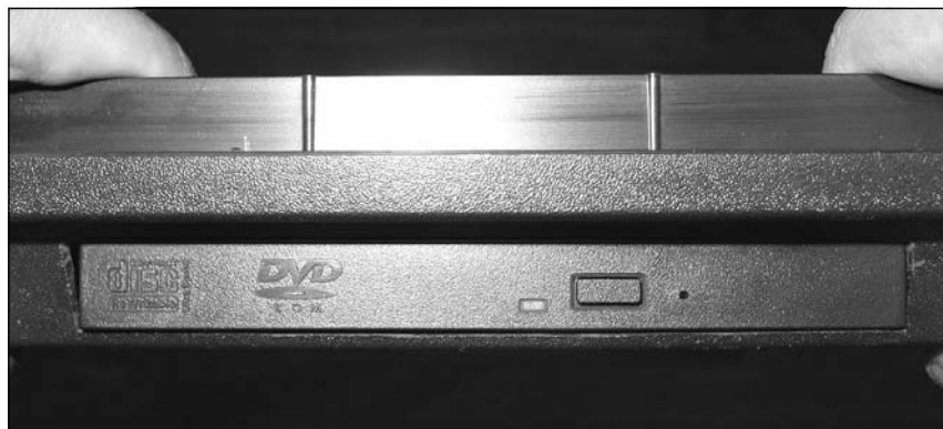
Figure 2.56 The Completed CD-ROM/DVD Drive Slot
