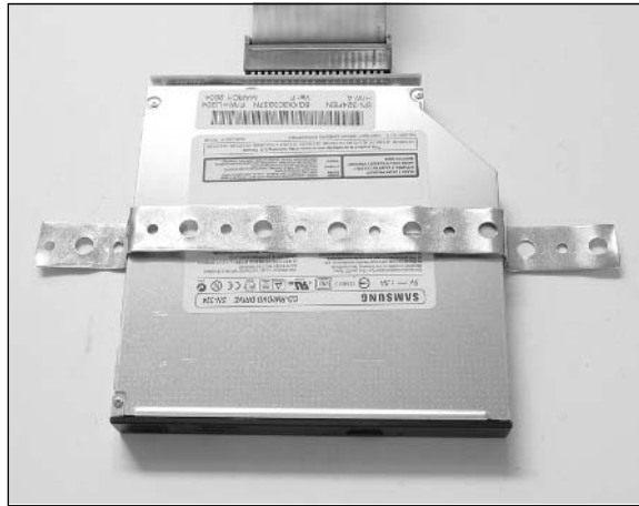
Figure 2.66 The CD-ROM Drive with Hanger Strap “Drive Rail”
