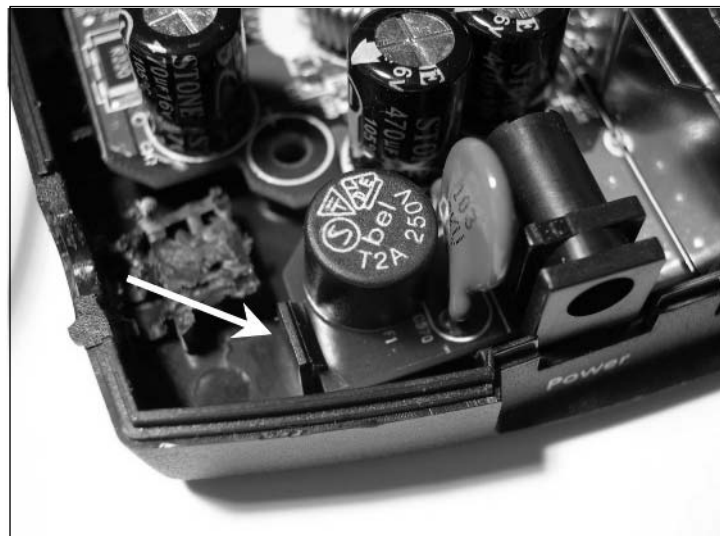
Figure 3.38 Clips to Hold the Circuit Board
