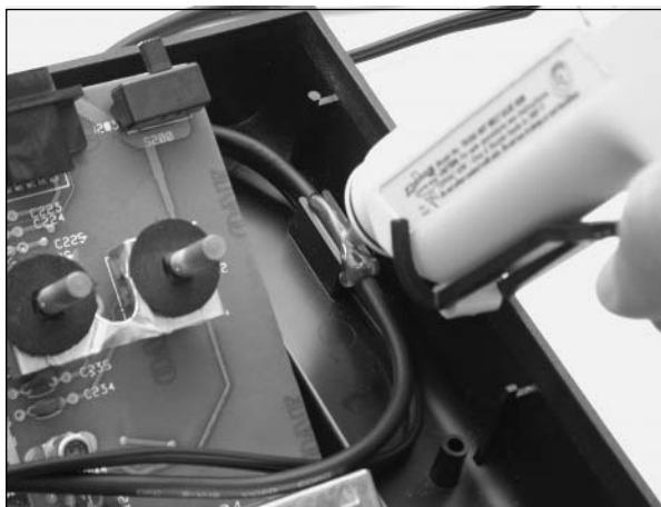
Figure 8.72 Securing the Cables, Continued (Optional)
