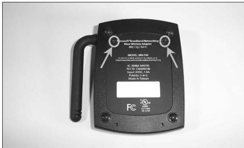
Figure 3.36 The Bottom of the Xbox Wireless Adapter Showing the Case Screws
