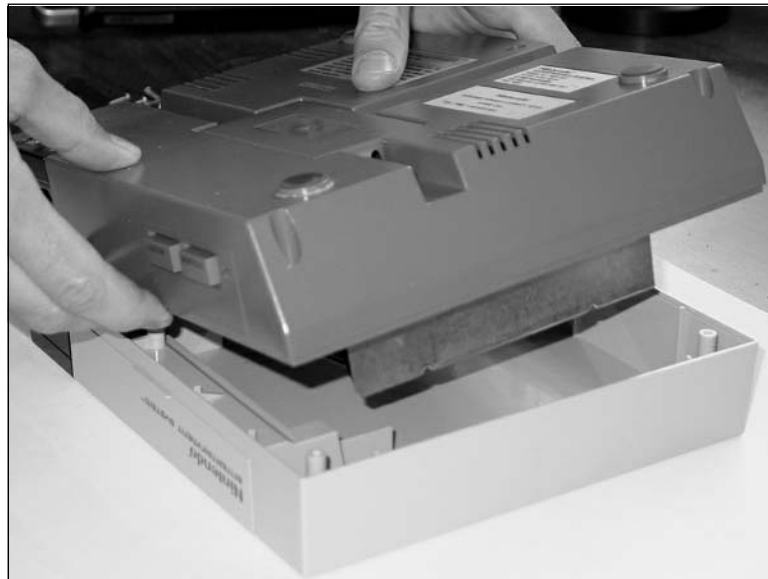
Figure 7.5 Separate the Bottom and Top Halves of the Console
