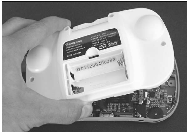
Figure 6.14 Separate the Bottom and Top Halves of the Console
