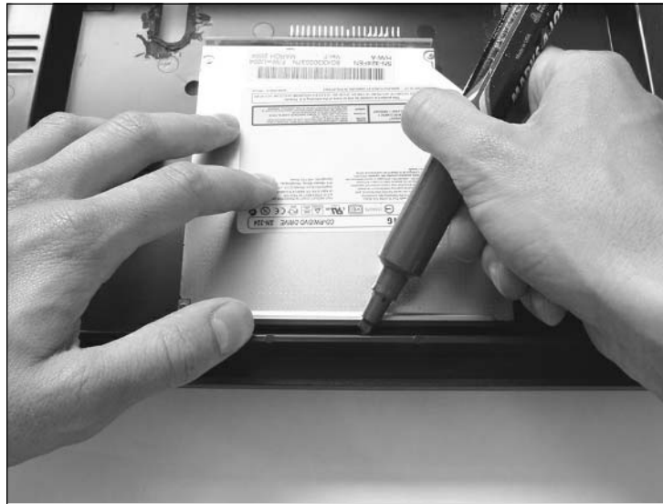
Figure 2.55 Marking the CD-ROM/DVD Drive Tray Location on the Atari 2600 Bottom Housing
