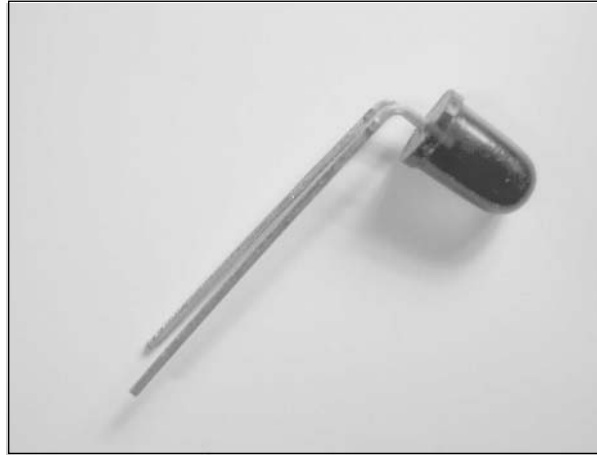
Figure 3.15 LED Leads Bent 90 Degrees
