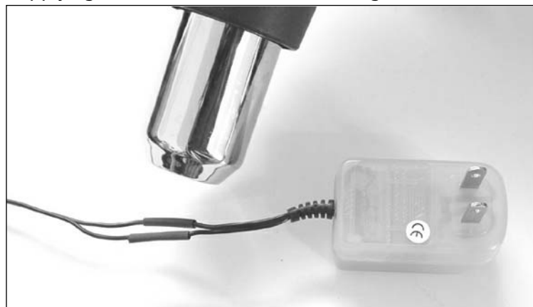
Figure 6.45 Applying Heat to the Heat-Shrink Tubing
