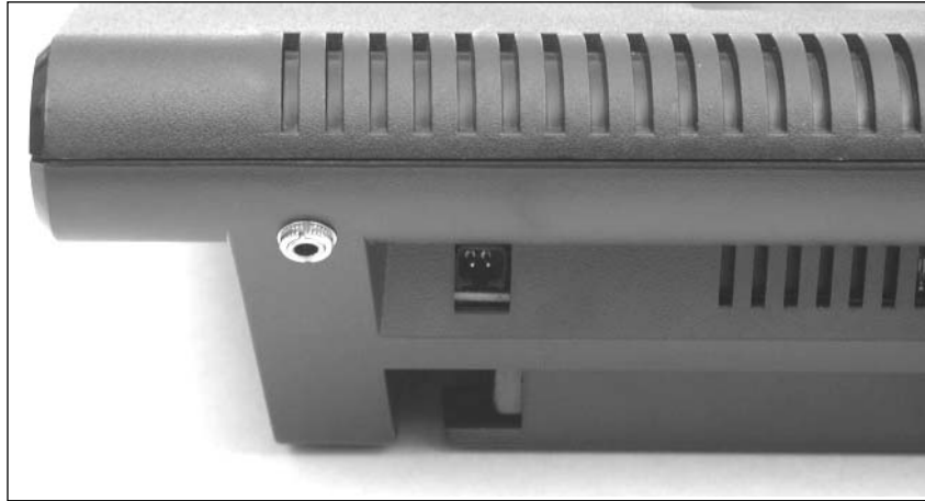
Figure 10.29 Back of the Atari 7800 Showing the New Power Jack
