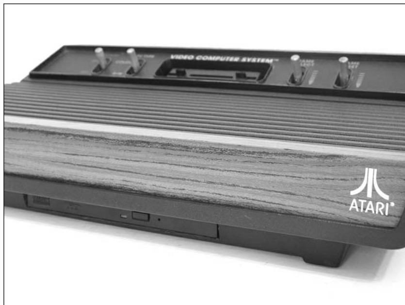
Figure 2.84 The Completed Atari 2600 Case Mod: Close-Up Showing CD-ROM Drive
