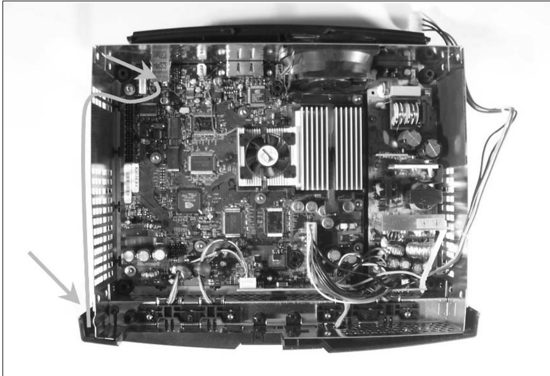
Figure 3.33 Run the Wires from the Front Panel to the Ethernet Port
