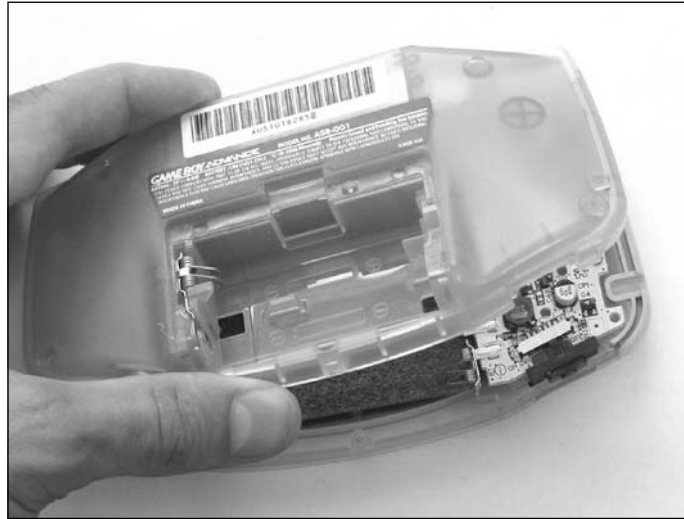
Figure 5.7 Separate the Bottom and Top Halves of the Console
