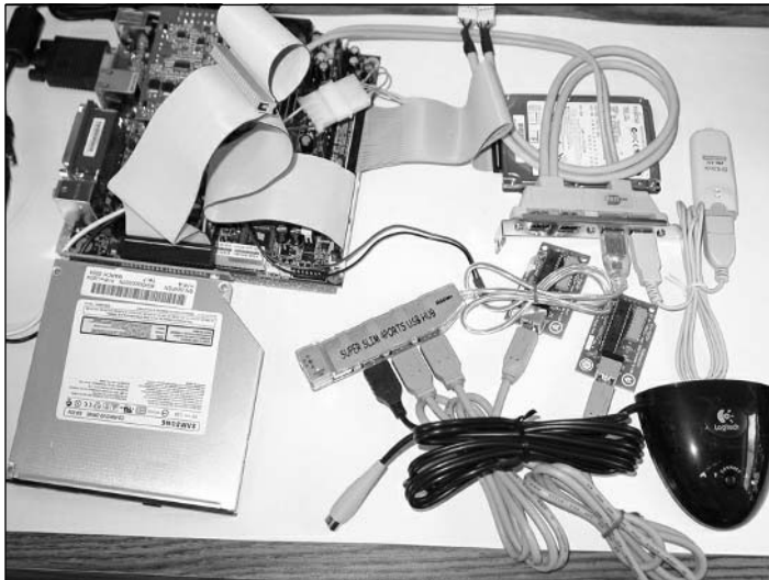
Figure 2.13 Connecting All the System Components
