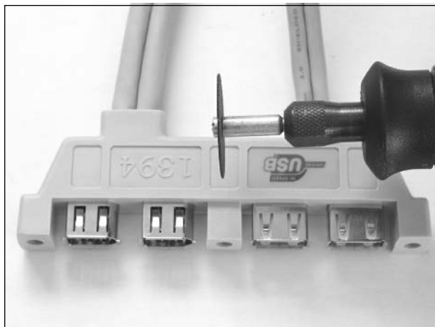
Figure 2.30 Removing the Unneeded Parts from the Backplane
