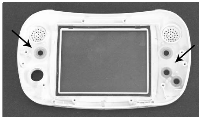
Figure 6.32 GP32 Top Housing Showing Button Membranes
