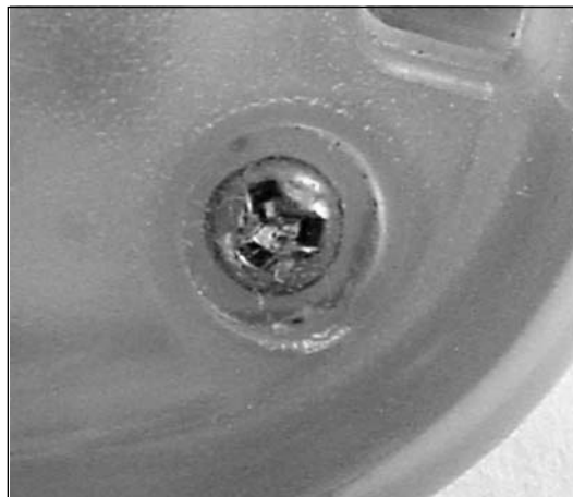
Figure 5.5 Close-Up of the NES Tri-Wing Security Screw
