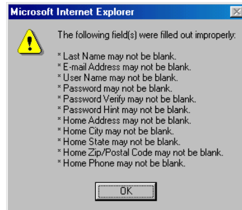
Figure 6: Page-by-page validation can make it difficult for users to manage a huge report of errors.
