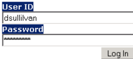
Figure 4.2: Masking the characters in passwords does not prevent password stealers, which detect characters as they are sent from the keyboard to the application.
