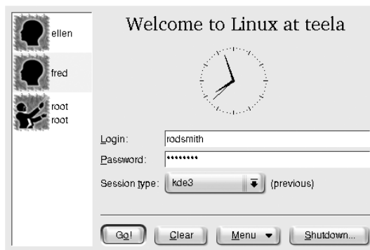
FIGURE 2.7 KDM, like GDM, enables users to select a desktop environment or window manager at login time.
