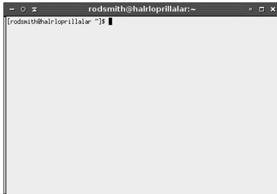
FIGURE 1.1 An xterm window enables you to type text-mode commands in a GUI session.
