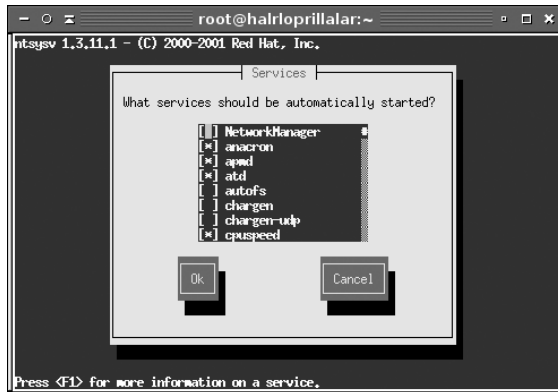
FIGURE 6.2 The ntsysv program enables you to control services from a menu of available services.
