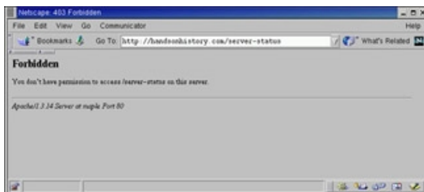
Figure 21-4: Deny server-status and server-info access to hosts on external networks, and perhaps to any machine other than the server.
