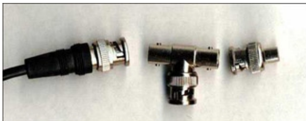
Figure 15-4: A bus topology has coaxial cables that must be terminated (as shown) or continued from the T.
