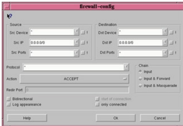
Figure 14–2: Clicking New on the main firewall-config window brings up a window for composing a new ipchain rule.
