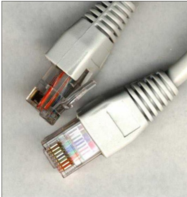
Figure 15-3: A star topology's twisted pair cables have RJ-45 connectors (similar to telephone cable connectors).
