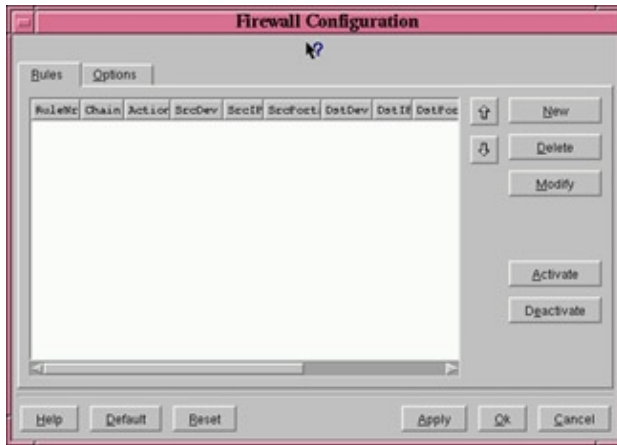
Figure 14–1: The main firewall-config window will display the list of all ipchain rules.
