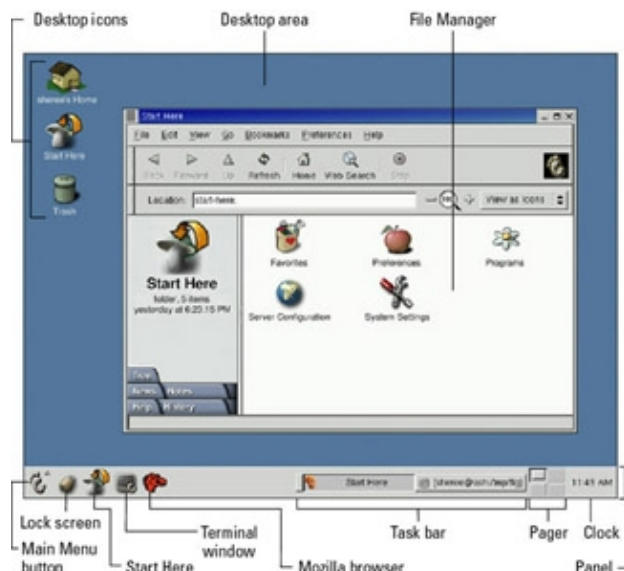
Figure 4–2: In the GNOME desktop environment, you can manage applications from the panel.
