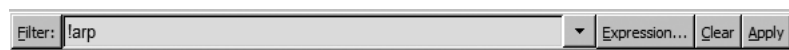
Figure 4-9: Creating a display filter using the Filter text box above the Packet List pane.
