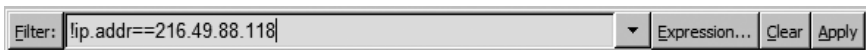
Figure 7-29: This filter removes all of the legitimate traffic so we can focus on what is abnormal.
