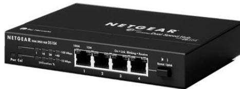
Figure 1-3: A typical four-port Ethernet hub
