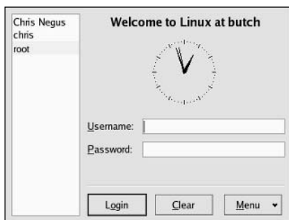
Figure 3-1: A simple KDE display manager ( kdm ) login screen includes a clock, login name list, and a few menu selections.
